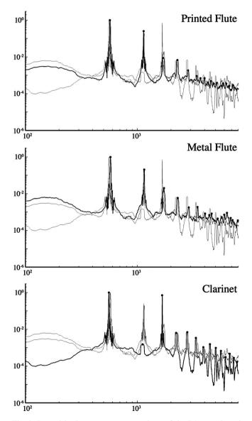
Fig. 8. Logarithmic spectrum comparison of the B1 note, based on recordings of a length of 0.3 s which do not include the transient, of a printed Objet's flute (top), a regular metal flute (middle), and a clarinet (bottom). In each plot the grey graphs are the two other recordings, for reference. The clarinet sound sample was taken from www.compositiontoday.com, and was not recorded under the exact same conditions.
