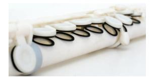
Fig. 7. A picture of the Objet flute's printed pads (soft material in black), printed simultaneously with the flute body and key mechanisms (rigid material in white).
