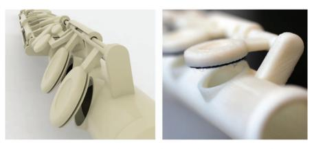
Fig. 4. The design of the printed plastic pads (left), and a picture of the glued felt solution (right) for the FDM flute. The computer rendering in the left was made using V-Ray software.
